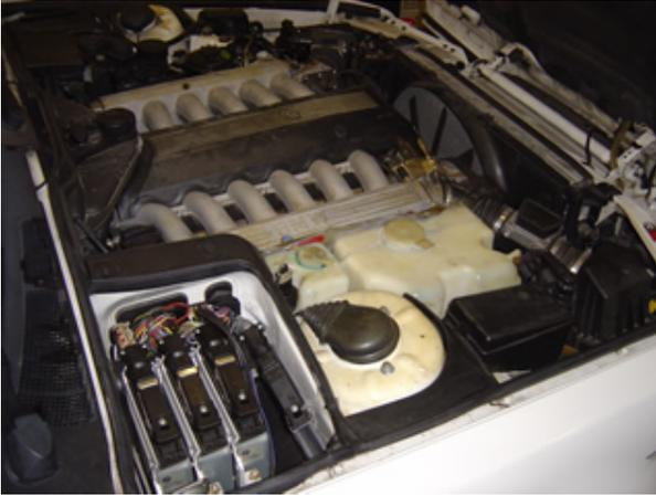
Easier said than done, usual time with being careful is about ten to fifteen hours for a novice. Disconnect all cables, labelling those going to your ignition coils, crank sensors, air mass sensors and DK motors. You will need to record the position of these sensors and actuators to ensure you do not get the banks crossed over when it comes to reconnect everything. Before you start work, disconnect the battery.
