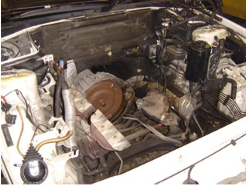
*Engine bay after loom and engine removal*
