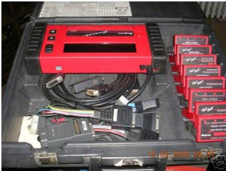
*This is the Snap-On MT2500 scanner I used to debug my system. Any code reader capable of reading a BMW 7 or 8 series can be used, although the better ones like this, allow you to test certain parts of the system such as the fuel injectors and can give valuable diagnostic information*
